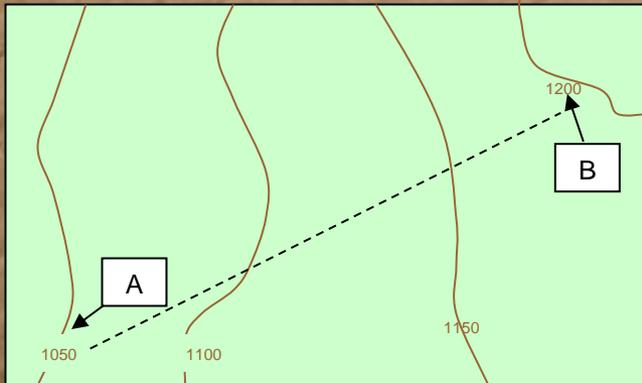
The climb from point A to point B is 150 feet (vertical) – the gradient is moderate as indicated by the contours being reasonably far apart. In real life the gradient would look that that shown below.
