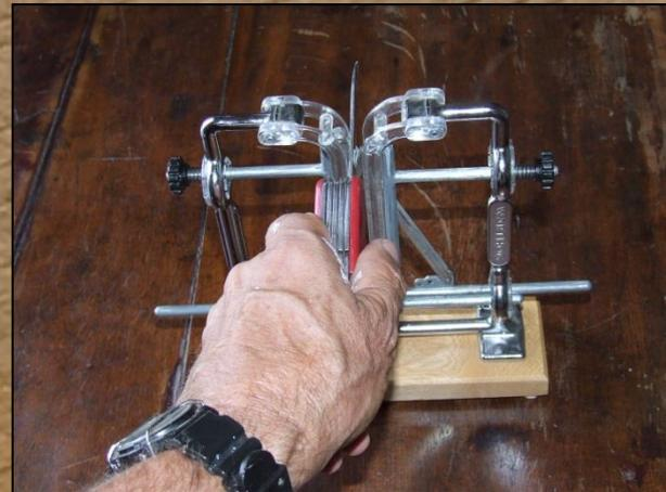
When using a commercial knife sharpening device like the “Warthog” (above right) the knife blade is drawn through ceramic rods that are tensioned up against the blade with springs. A “Lansky” knife sharpener supplies stones of various grit and a knife holder that holds the blade at a specific angle. Sharpening begins with a coarse stone working down to finer grits.
