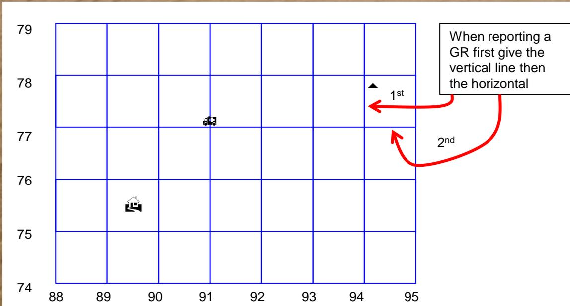
The Grid Square in which the black triangle is located would be indicated by the grid lines 94 (vertical) and 77 (horizontal). We can say the black triangle is in grid square 9477. This is a 4 figure GR.
