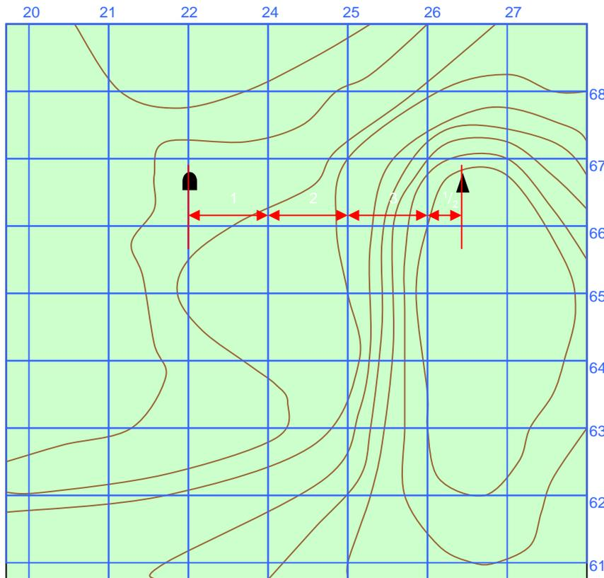
If we know the scale of the map (e.g. 1 grid square is equal to one square km) then by counting the number of squares we can determine the distance between two points.
