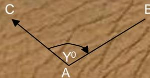
A magnetic bearing is taken from point A on the ground to point B. The angle  $y^{\circ}$  is measured clockwise from AC to the line AB.
