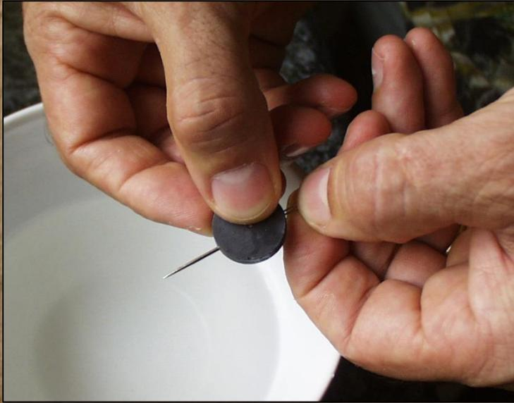
Magnetizing a compass needle with a magnet or satin cloth and then floating the needle on a leaf in some water makes a functional compass.
