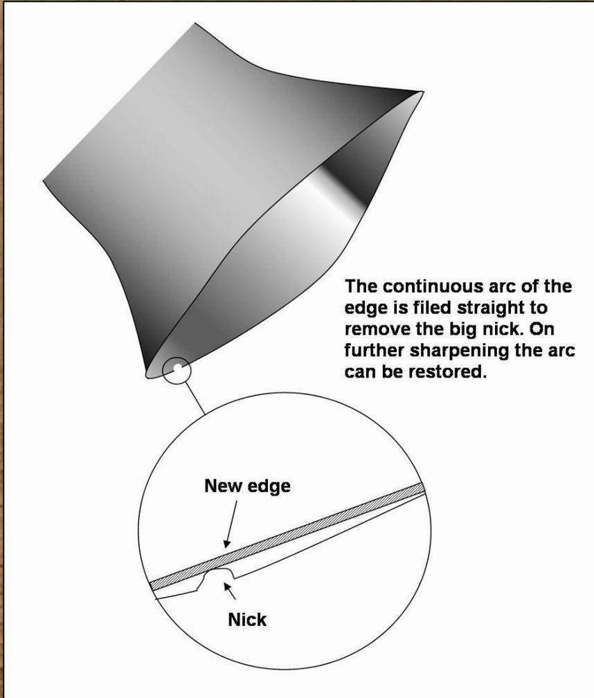
Experienced axe users file the axe towards the blade as this ultimately provides a better blade shape and thinner edge burrs. See next page. Filing in the same direction as the cutting edge is however a safer option.
